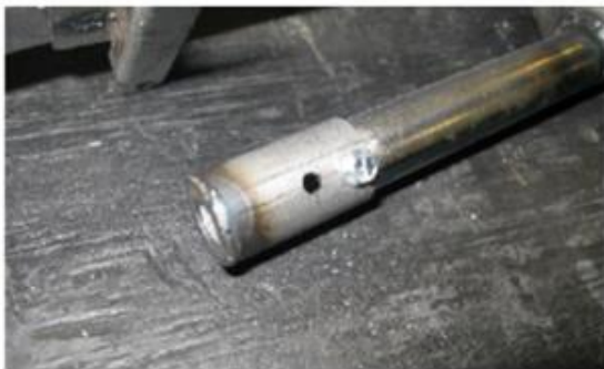
NG Air Collar Installed
