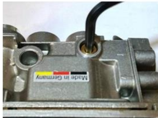
Location of Low Pressure Adjust Screw (Under the fireplace)
